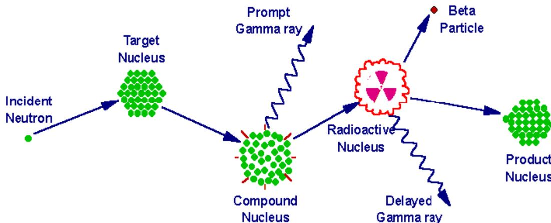
Fig. 15.4 Incident neutrons irradiate target nuclei in an unknown sample to form a compound nucleus, which emits a prompt gamma ray to produce a radioactive product nucleus. The decay of the product emits beta particles and gamma rays that can be used as fingerprints of the product  $A + 1$  nucleus. Because neutrons do not increase the atomic number, identification of the product defines the element and isotope(s) of the constituents of the sample.
