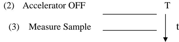
In step (1) (accelerator on) the product is being produced and undergoing decay simultaneously. Step (2) (accelerator off) involves only decay of the sample after the irradiation has ceased. Step (3) involves measurement of the sample as it decays away according to the first order decay law.
