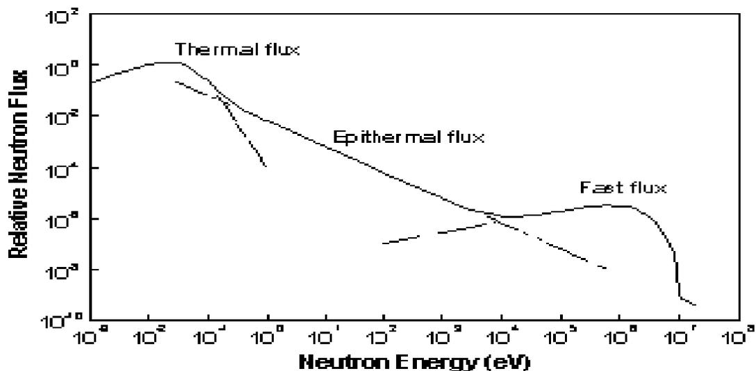
Fig. 15.5 Three major neutron flux distributions in a nuclear reactor: thermal flux, corresponding to room temperature velocities (meV); epithermal flux at intermediate energies (eV – keV), and fast flux due to fission reactions (keV – MeV).
