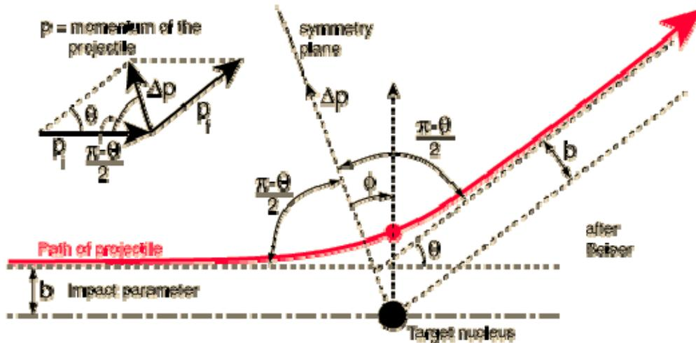
Fig 15.2 The Coulomb trajectory of a projectile incident upon a target nucleus, where  $\theta$  is the angle of deflection from the incident path;  $b$  is the impact parameter, the distance from the trajectory that coincides with the center of the target nucleus and  $\Delta p$  is the momentum change. It was this sort of analysis that led Rutherford to deduce the size of the nucleus.
