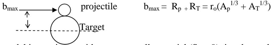
Such a model is consistent with a square-well potential (Sec. 9): i.e. the nuclear force is either on or off. Thus if the target and projectile touch ( $b \leq R_p + R_T$ ), there is a reaction. If  $b > R_p + R_T$ , then there is no reaction. The probability that the projectile will hit the target is given by the cross-sectional area defined by the two touching spheres, called the **total reaction cross section**  $\sigma_R$ , where
