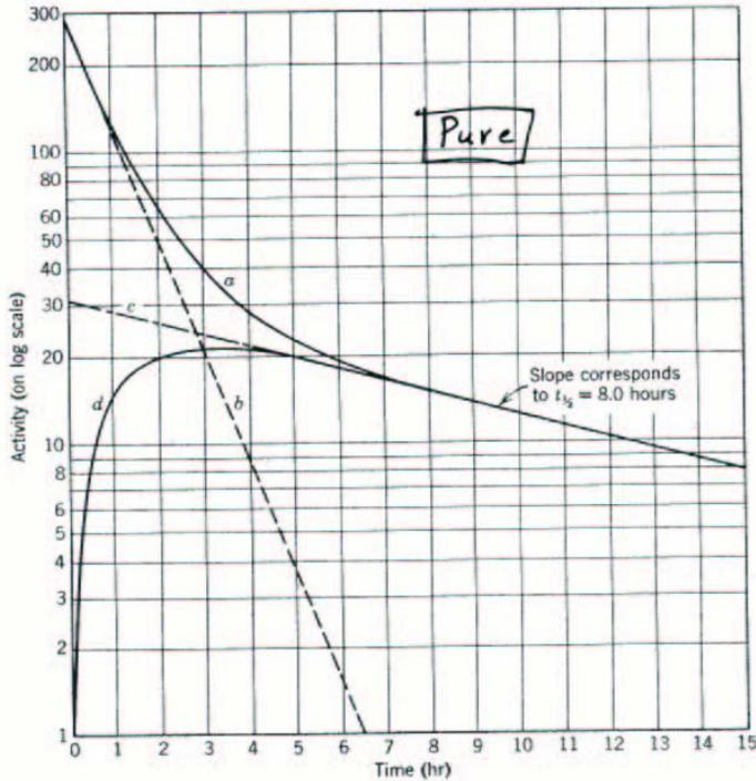
Fig.14.4 Example of no equilibrium: total activity (curve a); growth of daughter activity (curve d); long-time behavior of daughter (curve c), extrapolated to time = 0, and decay of parent (curve b).
