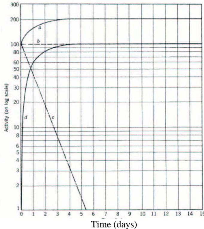
Fig. 14.6 Parent-daughter behavior for secular equilibrium: total activity (curve a); parent decay (line b); growth of the daughter (curve d), and the independent decay curve of the daughter (curve c).
