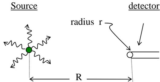
Fig. 14.2 Schematic diagram of a radiation detection measurement in which a detector of radius r intercepts radiation at a distance R from a radioactive source.
