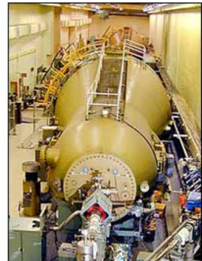
Tandem accelerator at Brookhaven National Lab. (BNL)
